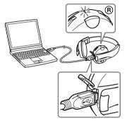
Charging starts when the unit and the computer are connected. Make sure that the indicator (red) lights up. Charging is completed in about 4 hours\* and the indicator (red) goes off automatically.
